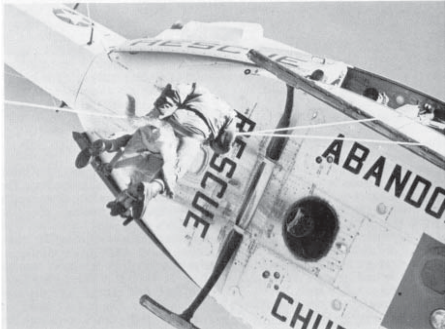
After clearing the skid, the handler "rides" the dog down. Note the safety belay line as well as the rappel rope. Credit: Official Navy photos by PHI Ron Mathews.
